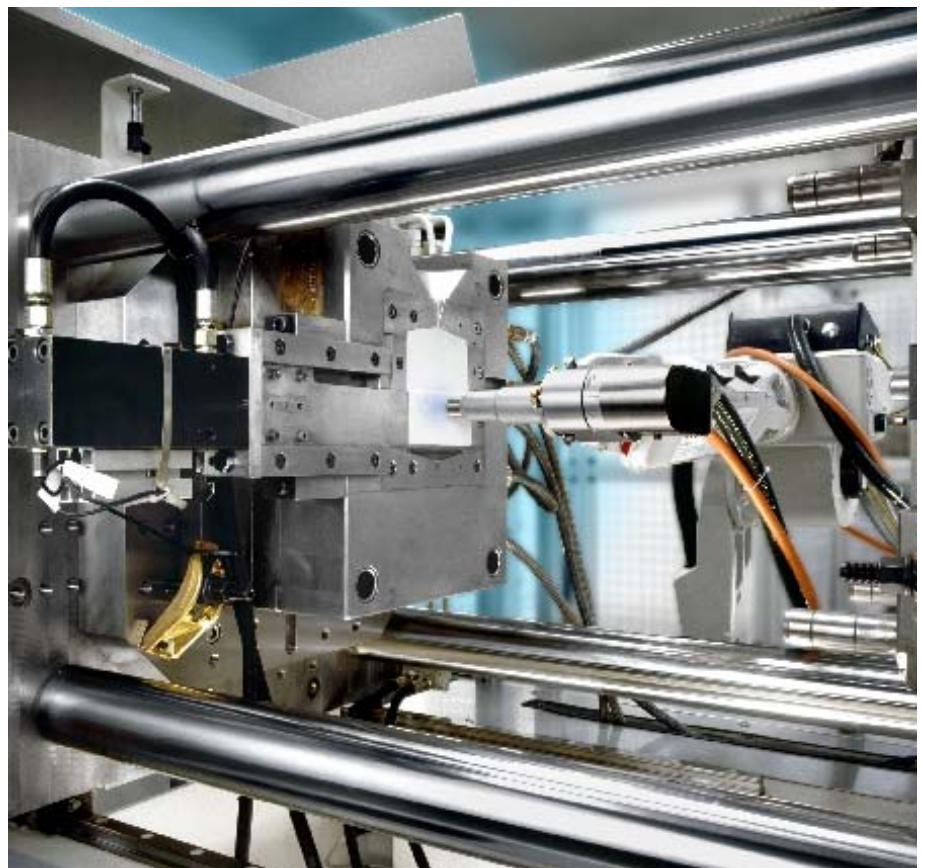
When the mould is opened a bending arm robot moves the plasma jet up to the contact surface of the injection moulded part.
