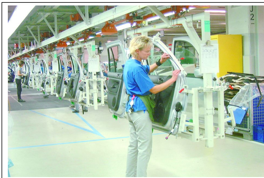
Source: Plasmamatreat with authorization of VW Figure 6: In the meantime almost all door production lines at Volkswagen have been equipped with the Openair Plasma pre-treatment system.
