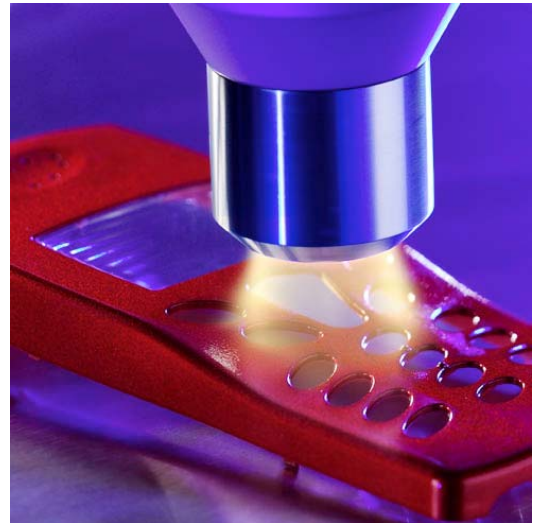
The mobile phone housing is cleaned by a rotating plasma jet prior to painting
