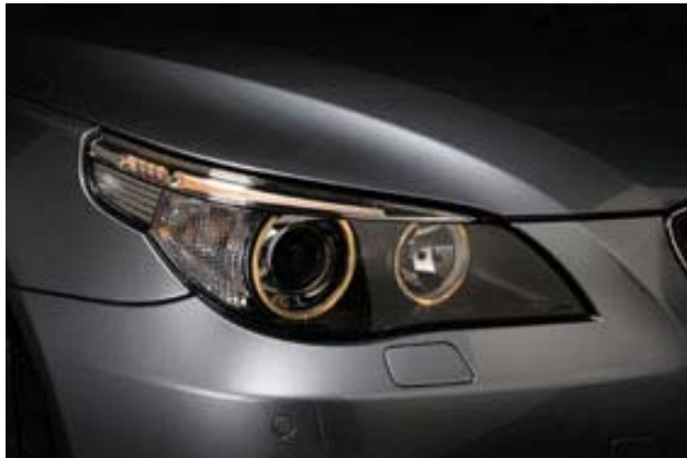
Pretreatment with plasma is also used in the painting of headlight lenses
