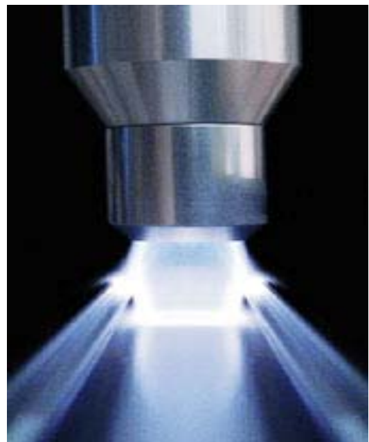
An atmospheric pressure plasma is generated inside the plasma jet by means of high-voltage discharge
