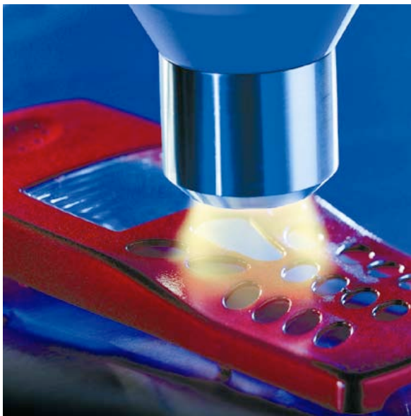
Fig. 6: Pretreatment with Openair plasma ensures ultrafine cleaning of mobile phone housings prior to painting
