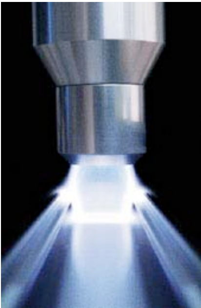
Fig. 3. The electrically neutral plasma beam allows ultrafine cleaning, high activation and wafer-thin coating of surfaces
