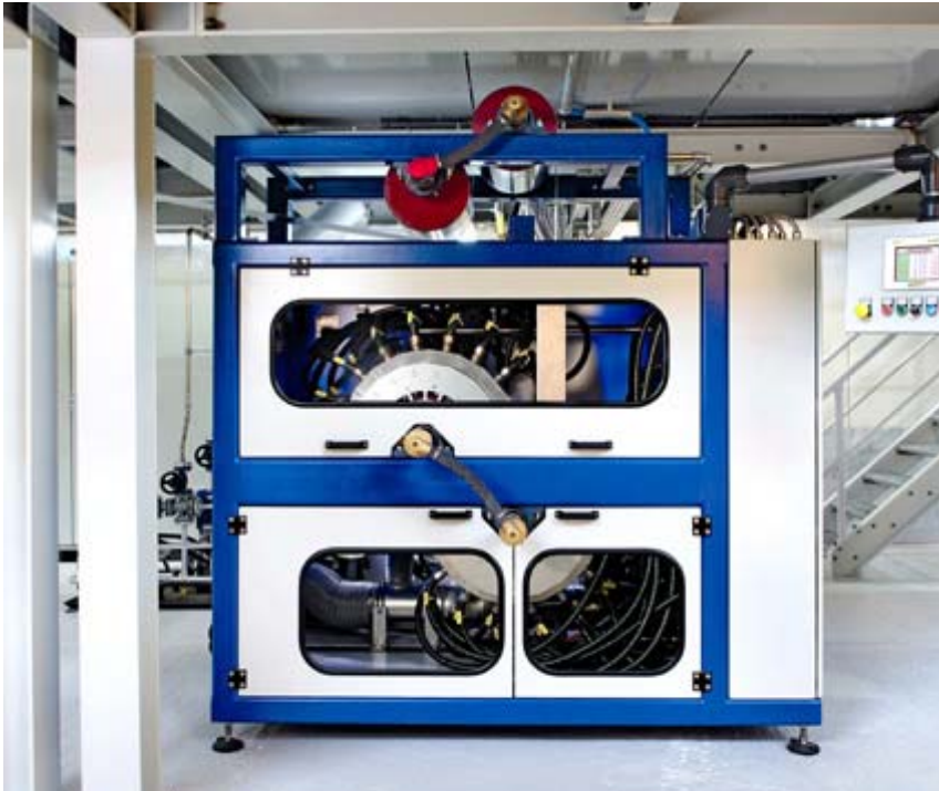
The use of plasma in the coil coating process is unique anywhere in the world. The plasma installation measuring only 2 x 1.5 m replaces a 21m long cleaning line.
