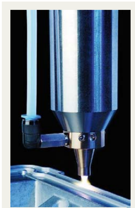
Photo Plasmatreat Coating by means of atmospheric-pressure plasma can be integrated in ideal fashion into existing production systems for aluminium parts
