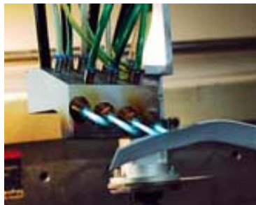
The dismantled plasma jet: Flames softening the adhesive of the hand-held edge (Photo: G.Molinski, dds)
