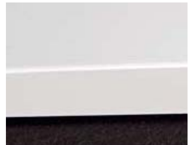
Zero-joint, heat-resistant and humidity-resistant up to 140 °C: Plasma-abutted edge (Photo: R. Schumacher)
