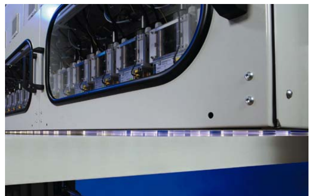
FIG. 7. 28 rotary nozzles, each designed for a treatment width of 100 mm, are arranged in two rows and offset from one another. In this way, up to 3 m wide panels can be activated and cleaned to a microfine level (all figures: Plasmatreat).
