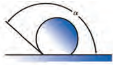
Poor surface wetting
