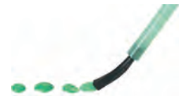
Poor surface wetting
