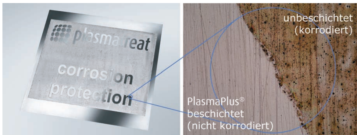
Fig 3: The plasma-polymer coating not only serves as an excellent adhesive substrate; by acting as a barrier against corrosive electrolytes it also provides exceptional corrosion protection.
