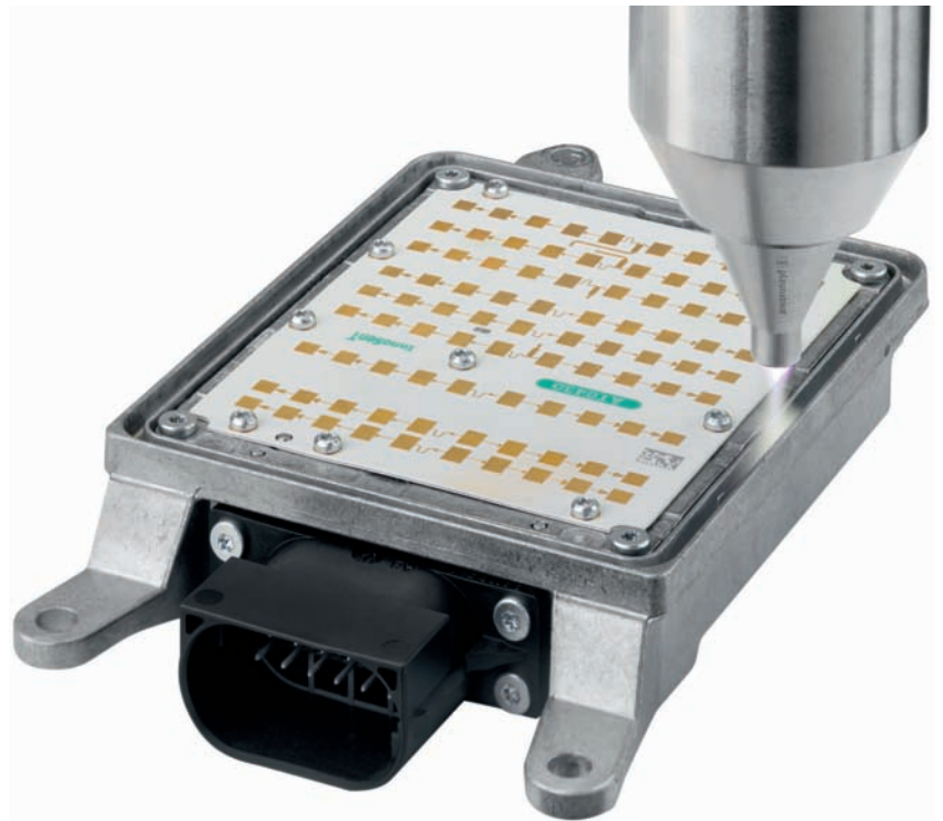
Fig 2: The plasma beam impinging on the surface at high speed removes all organic impurities from the metal and restores its surface energy.
