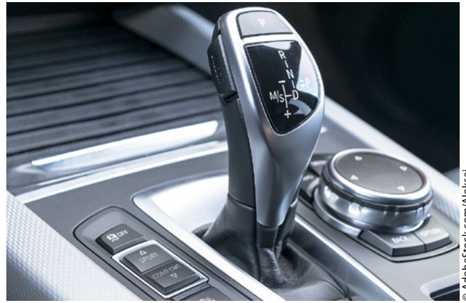
A plasma treatment enhances the durability of coatings and printed lettering on the control elements in the vehicle interior.
